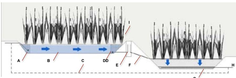
Figure 1 - Horizontal Subsurface Flow Wetland (left), Vertical Flow Subsurface Wetland (right)
