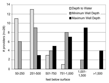
Figure 8. Depth to Water, Minimum and Maximum Well Depths.
