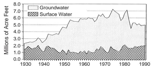
**Figure 2.4.** Surface and Groundwater Annual Extraction: Arizona, 1930 to 1990. Source: Arizona Department of Water Resources (1994b).
