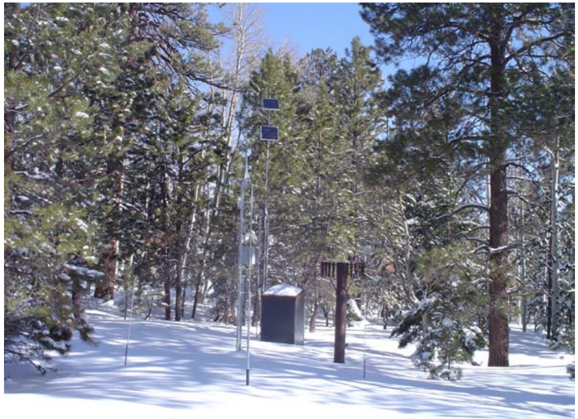
Figure 1. The Beaver Spring SNOTEL site is located in northeastern Arizona near the border with New Mexico. Most SNOTEL and snow course sites are located at high elevations and in clearings where tree canopy does not obstruct precipitation. A typical station contains a rain gauge (the rusty-looking feature in the photograph), solar panels, weather sensors, and a snow pillow (outlined by the three visible poles in the foreground). Photograph courtesy of Dino De Simon, NRCS.
