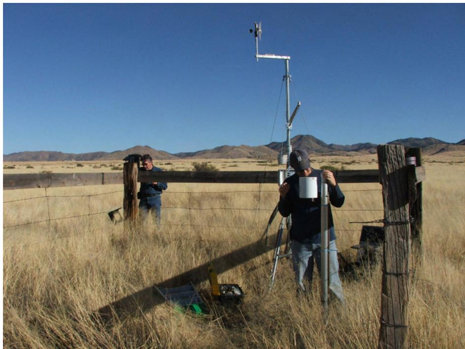
**Figure 2:** UA scientist Mike Crimmins peers into a rain gauge, while colleague Wim van Leeuwen adds a larger memory card to the self-timed, digital camera.
