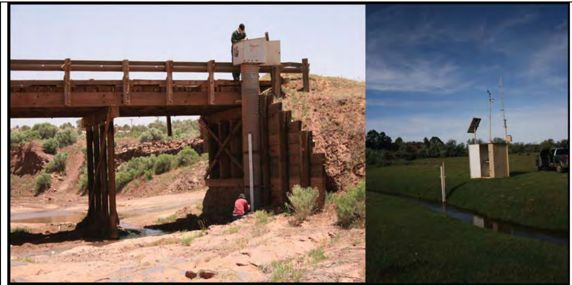
Figure 6.5. Stream flow gaging station locations for Kinlichee Creek (left) and Tsaile Creek (right). Note that these two streams have different gage types: a stilling well in Kinlichee Creek and a pressure transducer in Tsaile Creek.
